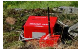
Example of a process warning system: geophone
