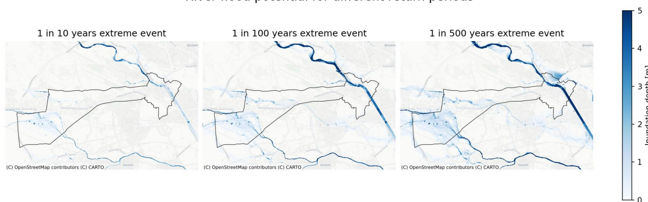
Figure 2 - 1 Flood extension and depth for the return periods of 10, 100 and 500 years.
