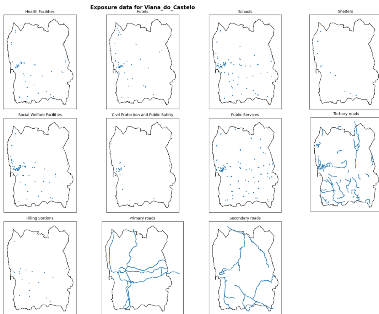
Figure 2-13 Detailed municipal exposure network including 11 critical infrastructure layers
