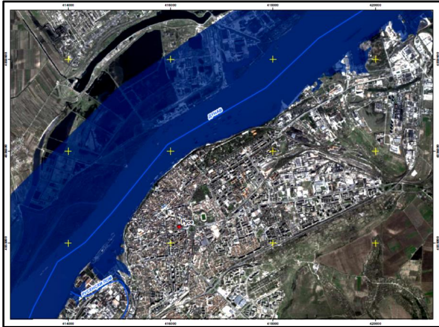
Figure 2.21. Sample map of flooded areas when simulating a wave height of 5m in transport corridor 7 and the Danube River – Ruse (Source: ReSak )
