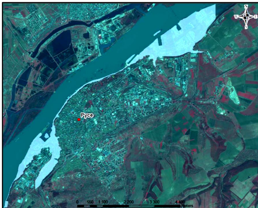
Figure 2.22. Sample map of flooded areas when simulating a wave height of 10 m in transport corridor 7 and the Danube River – Ruse (Source: ReSak )
