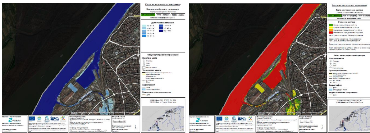
Figure 2.12. Flood depth and hazard, rcp20 (Source: Danube River Basin Directorate).
