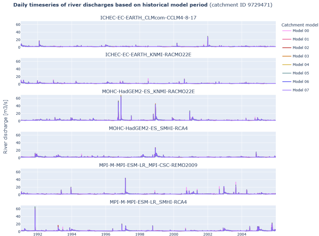
Figure 3: Daily timeseries of river discharges (m 3 /s) based on six (6) different GCM-RCM climate model combinations for the period 1991-2006.
