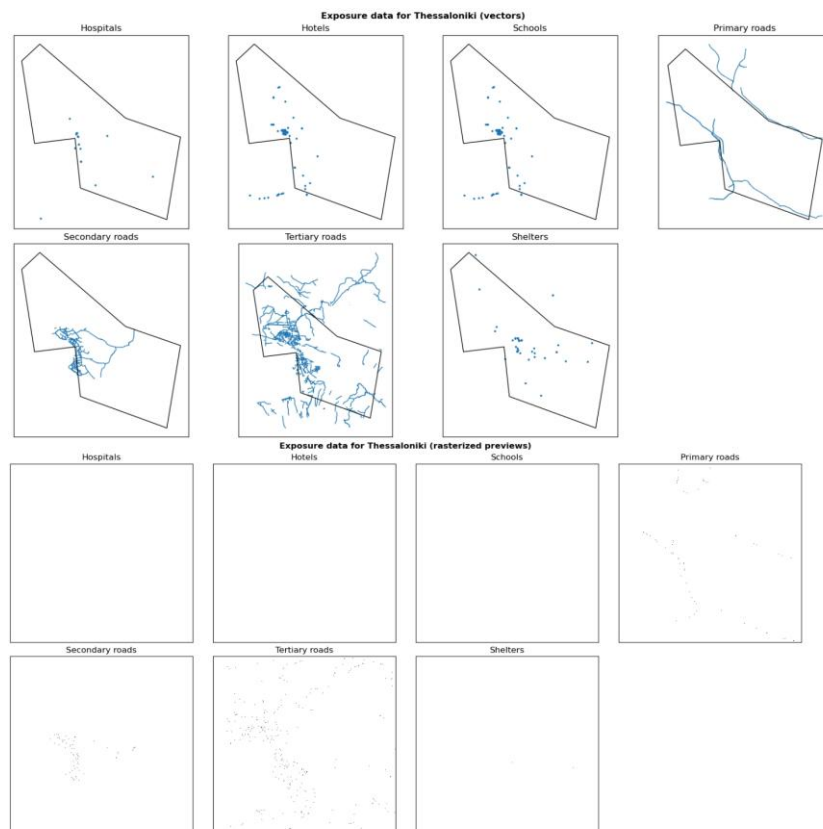
Figure 50: Exposure datasets for Thessaloniki used in the risk analysis, shown as (top) vector layers and (bottom) rasterized previews within the study-area boundary, including point-based assets (hospitals, hotels, schools, shelters) and road network classes (primary, secondary, and tertiary roads).
