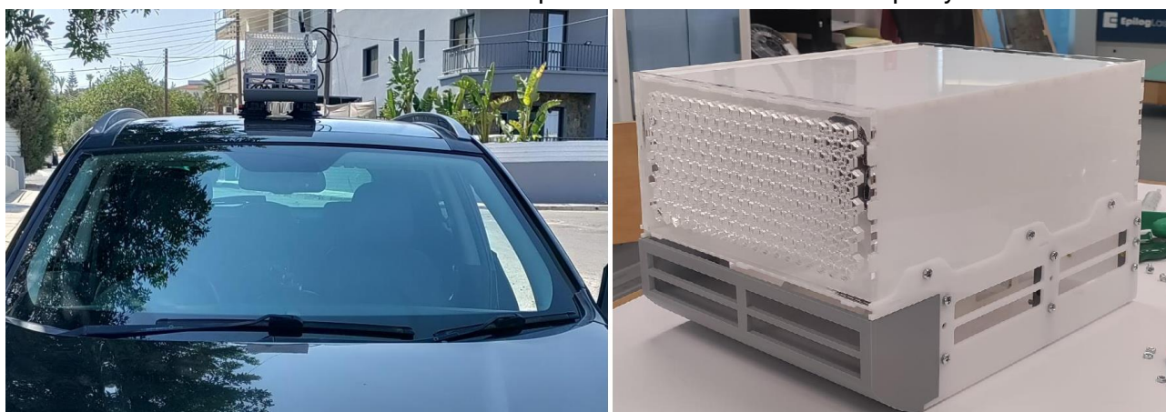
Figure 2-11. The equipment developed for studying the UHIE in Nicosia (right) and a demonstration of its mounting on a car for mobile use (left).
