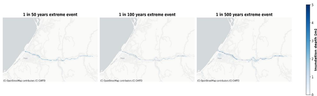
Figure 12 River flood potential for different return periods (Pixel size 9.2 x 9.2 m)
