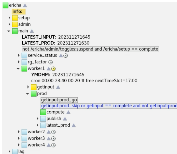
Figure 2. The ERICHA forecast product generation suite which is currently running at ECMWF. This structure will be adapted to integrate the tasks to generate the additional EDERA storm impact products.
